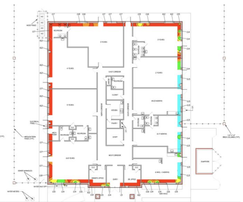
Figure 20.3 - Daycare Gypsum Sheathing Moisture Content Readings
