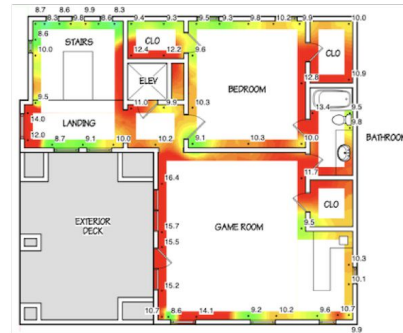
Figure 22.2 - House Baseboard Moisture Content Readings
