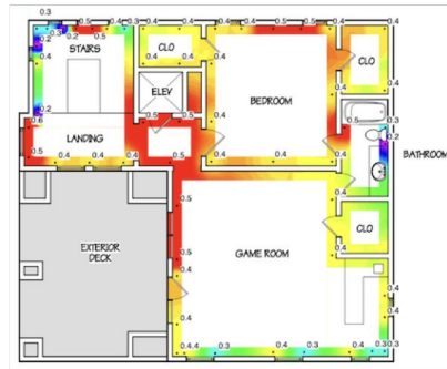
Figure 22.1 - House Gypsum Board Moisture Content Readings
