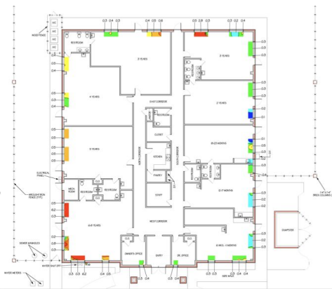
Figure 20.2 - Daycare Windowsill Moisture Content Readings
