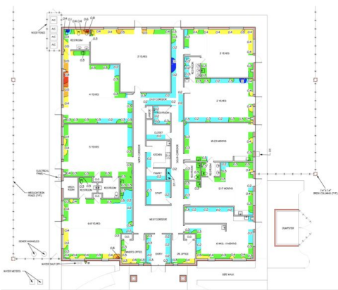
Figure 20.1 - Daycare Gypsum Board Moisture Content Readings
