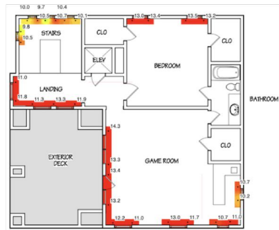
Figure 22.3 - House Door and Windowsill Moisture Content Readings
